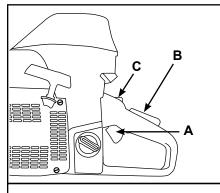
Figure 1: a-Trigger, b-trigger interlock, c-throttle lock
